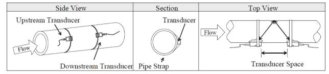
Z method installation on pipe size: 100mm to 3000mm
