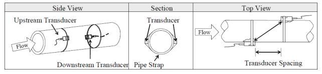
N method installation on pipe size: <50mm (Not recommended for most applications)
