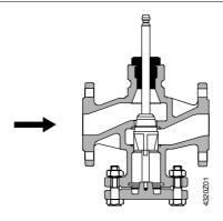
Guided parabolic plug, integrated into the valve stem.
