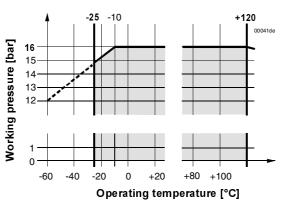
Working pressures classified to ISO 7268 and EN1333 at operating temperatures of – 25 ... +120 °C to DIN4747 and DIN3158
