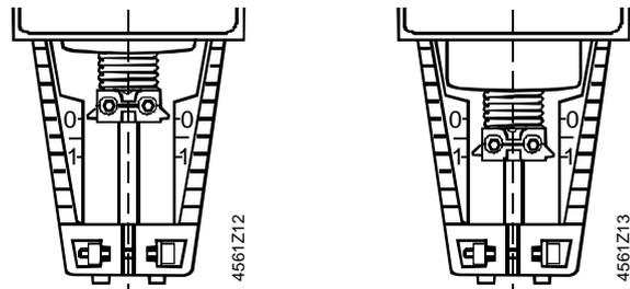
Coupling fully retracted → stroke = 0%      Coupling fully extended → stroke = 100 %
