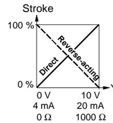
**Note** The mechanical spring-return function is not affected by the direction of operation selected.
