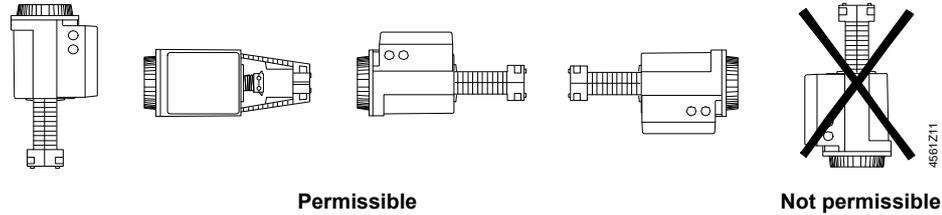
Instructions for fitting the actuator to the valve are bypacked in the actuator packaging. The instructions for accessories are enclosed with the accessories themselves.
