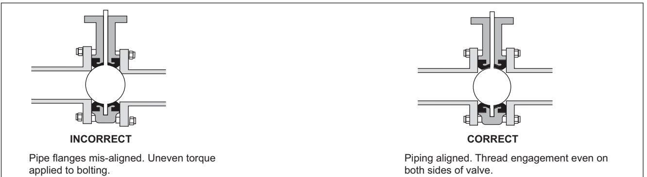
Figure 5 Installation notes for DN700..1200 BFV
