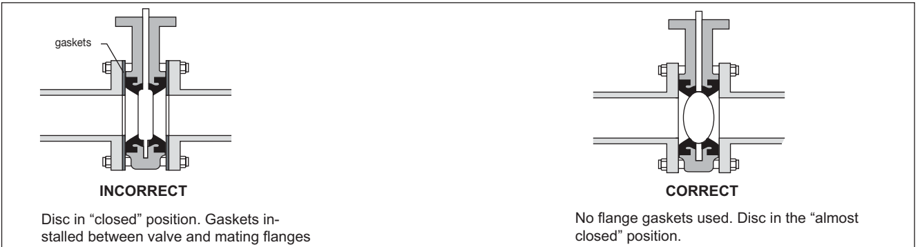
Figure 4 Final valve alignment and tightening of flange bolts
