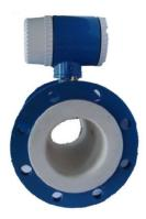
The shell of the flow sensor is welded with carbon steel. The electrode and lining only are in contact with the liquid media. The flow sensor and the converter may be one compact set or separately mounted.
